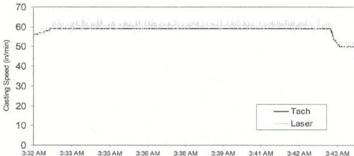
**Figure 6:** Speed Measurements. In this example which refers to a high casting speed situation, laser and tachometer speeds differ by approximately 2 ipm (i.e. a 3%-error for the current tachometer system).
