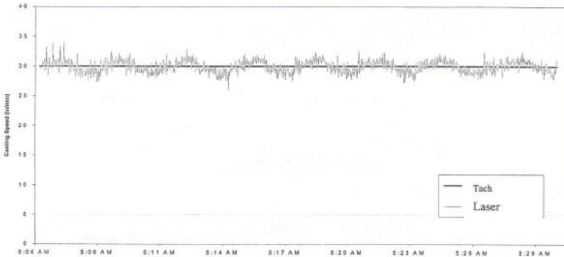
**Figure 9:** Preventative Maintenance. The unfiltered laser's output is much more variant than the tachometer's, and is so because of its precision. The caster does not run at a constant speed as the tachometer has always reported. Instead, casting speed changes all the time, in small amounts. Here, mold oscillations are very evident in the casting speed readout.
