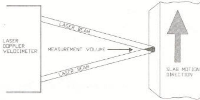
**Figure 1:** Principle of the Laser Doppler Velocimeter
