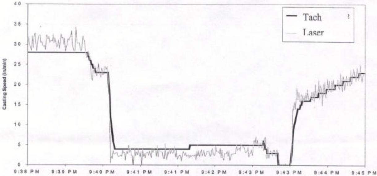
**Figure 7:** Speed Measurements. Even at slow speed (when there is less chance for roll slippage) the current tachometer has difficulty reading accurately.
