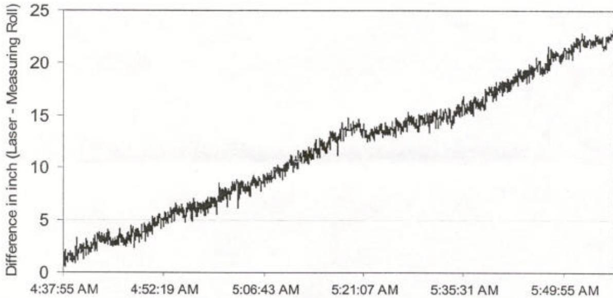
**Figure 8:** Length Measurements (Dec, 1, 2000 strand 2). The current measuring-roll system has accumulated a 22-inch error in less than 1:30 hours, i.e. approximately 2.2 inches/slab, equivalent to "losing" one slab/strand/day.
