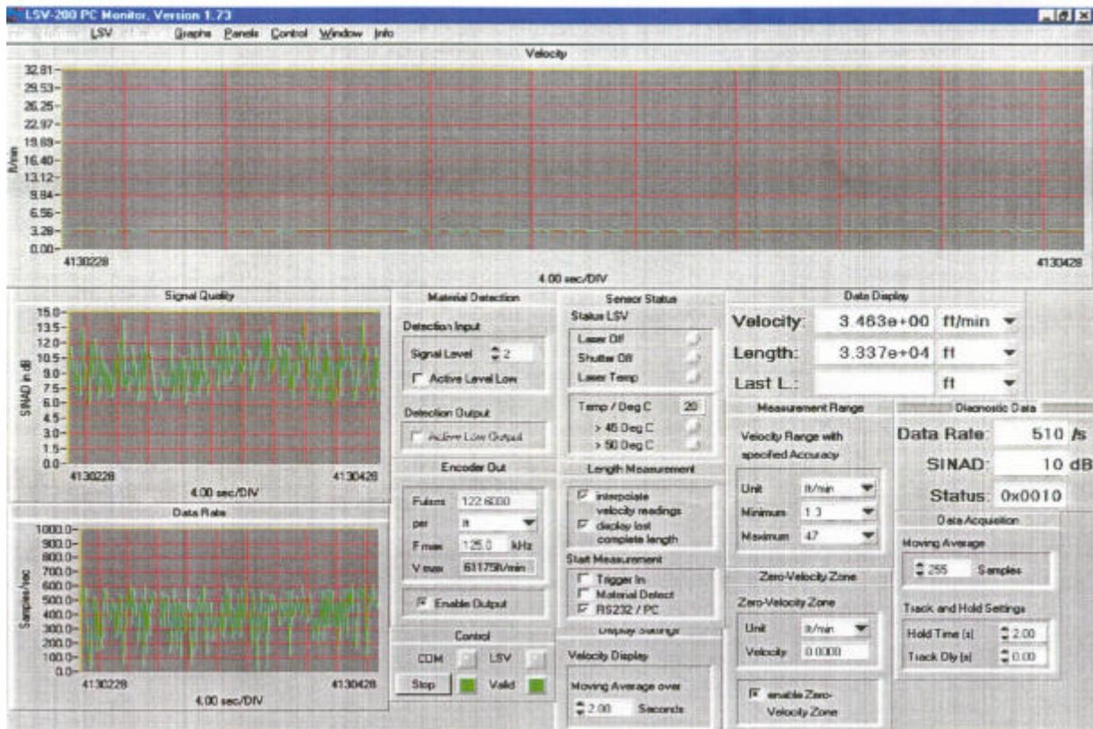
**Figure 5 :** Included with the Doppler system was software to adjust and monitor the equipment. The software monitors temperature with automatic shut-down capabilities, data rate from the Doppler's sensor head, signal quality, inch-count, and of course casting speed.
